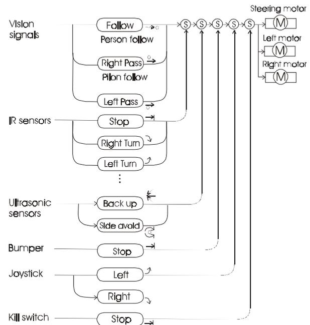
Figure 3.3 Software structure of M-2
