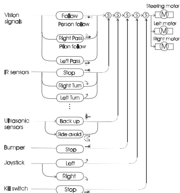
Figure 3.3 Software structure of M-2
