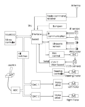
Figure 3.2 Hardware structure of M-2
