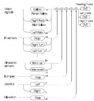
Figure 3.3 Software structure of M-2
